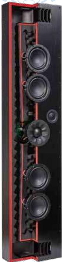
**ATL™** uses energy generated by the bass unit in a much more intelligent, efficient way than ported or sealed box designs. In **ATL™** loudspeakers, the highly braced cabinet is lined with specific acoustic materials that absorb all but the very lowest frequencies. These exit from a front vent extending the low frequency, all of which can be clearly heard at any volume level, from low to high.
