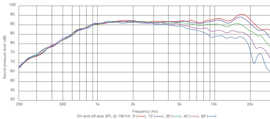
Figure 12: Axial response curve SPL v Frequency
