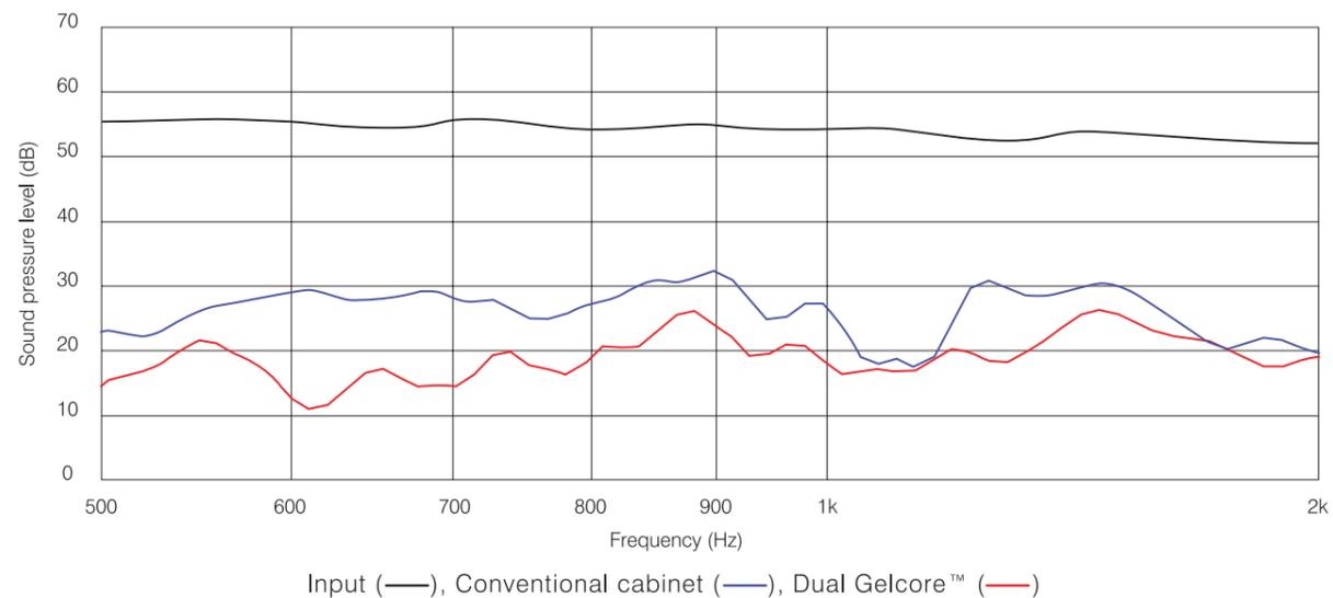
Figure 9: Graph to show SPL v Frequency for a conventional & Dual Gelcore cabinet wall
