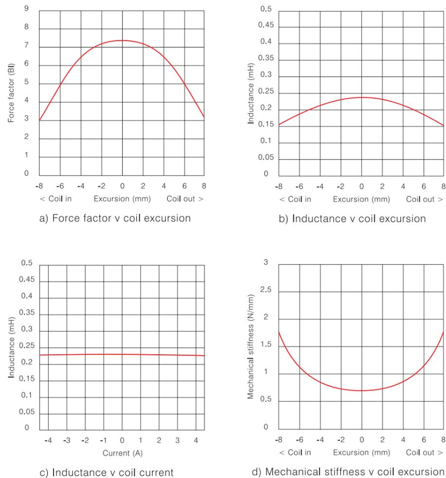
Figure 10: Mid/Bass Driver voice coil parameters
