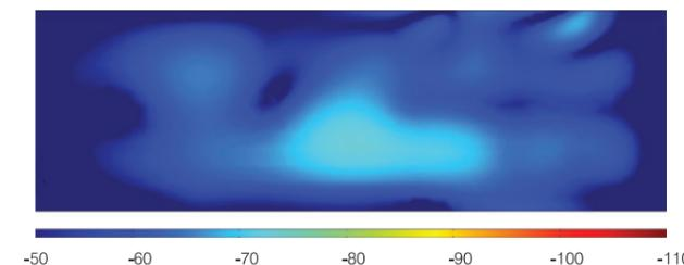
Figure 8: Heat map showing cabinet wall velocity with P2P Bracing
