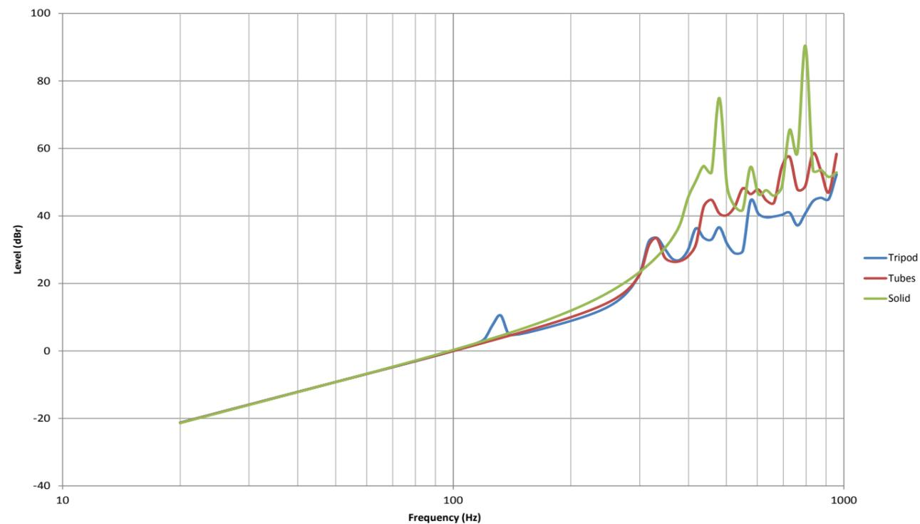
Figure 5: Normalised in-room acoustic power measurement for loudspeaker stands
