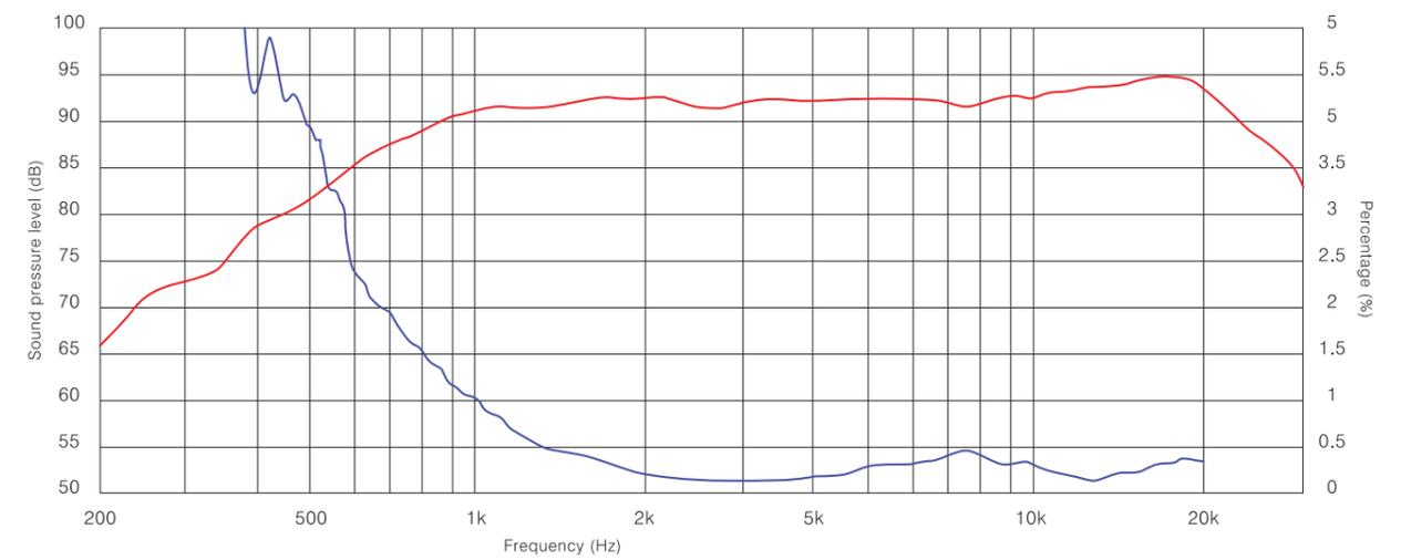
Figure 13: On-axis response curve high frequency drive
