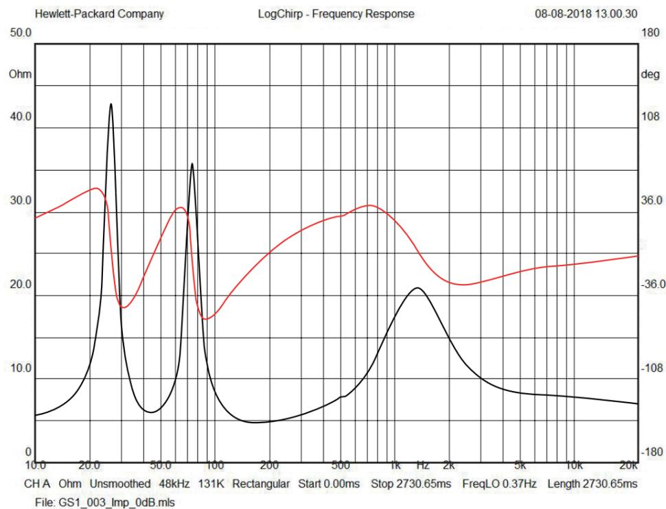
Fig. 14. Concept 300 Impedance/Phase Characteristic
