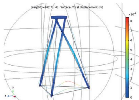
Figure 2. Total displacement Tensegrity Stand
