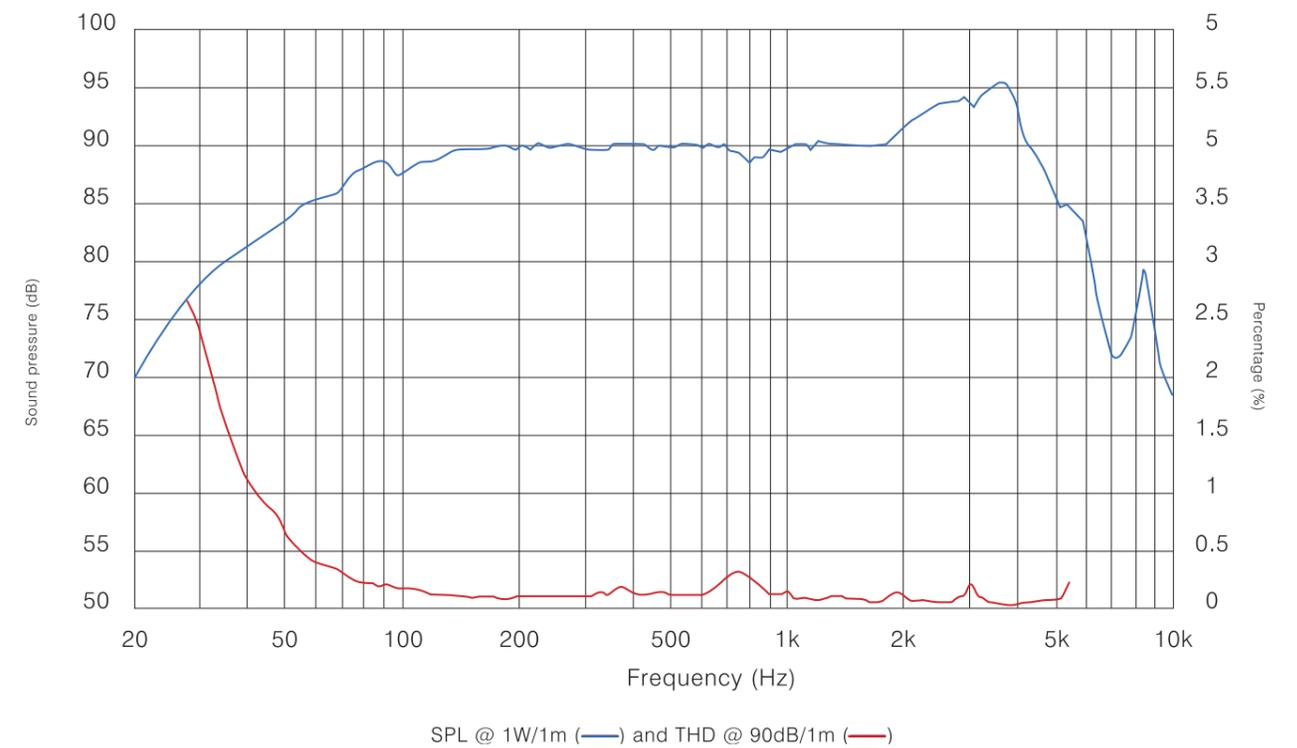
Figure 11: On axis response curve Mid/Bass unit without crossover
