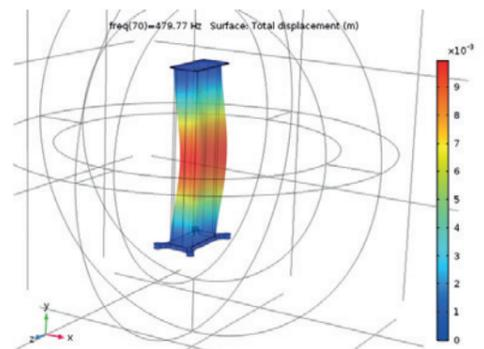
Figure 4. Total displacement Solid Stand
