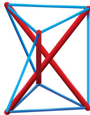
Figure 1. Tensegrity stand concept showing tension and compression elements
