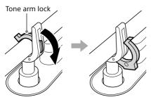
**5** Rotate the counterweight clockwise or counterclockwise until the tone arm is horizontally balanced.
