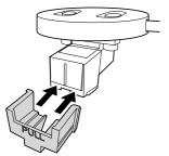
**3** Hold the cartridge body (1) with one hand, grasp the stylus with the other, and then pull the stylus in the direction of the arrow to remove it from the cartridge body.
