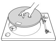
**5** Turn the platter upside down and remove the drive belt.
