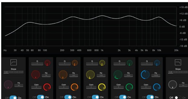
Frequency Response Graph (sample only to show response when you turn ON each parameter)
